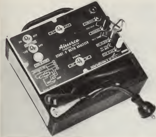
7-40. A capacitor test unit and analyzer. This unit will detect all hermetic and open motor troubles and can be used to reverse the motor. (Airservo Mfg. Co., Inc.)
